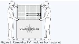
Check PV modules for damage due to transportation before they are installed; do not install damaged modules. Contact the company you purchased the Yingli Solar PV modules from in order to obtain information on making claims for defective PV modules.
