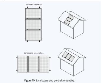
In order to maintain the fire class rating, the distance between the PV module bottom surface and the roof surface shall be at least 2.48 inches (6.3 cm). This spacing also allows air flow to cool the PV module. Install PV modules with a minimum spacing of 0.4 inches (1 cm) between neighboring frames to allow for thermal expansion.
