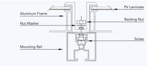
Figure 12: Detail of a top-down clamp mounting attachment
