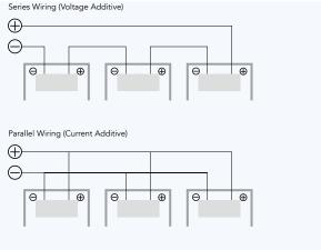
Figure 4: Electrical diagrams of series and parallel wiring
