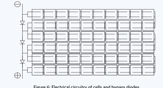
Figure 6: Electrical circuitry of cells and bypass diodes
