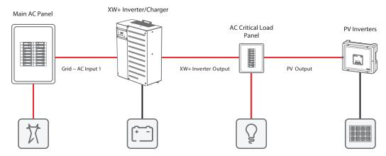
An example of AC Coupling with the Conext XW+ is shown in *Figure 1*. The PV system is connected to the grid through the internal relay located on the AC bus inside the Conext XW+ inverter. This allows power to be produced and supplied or "sold" back to the grid if it exceeds the power consumed by the critical loads.
