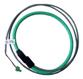
Self-powered rope CTs have a fixed amperage of 4800A. To configure a *self-powered* rope CT, select "RCT 152mm/5.98" 4800A" from the appropriate CT drop-down menu. Prior to firmware v2.16, choose "Rope 6" from the drop-down menu.
